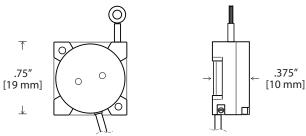
Introducing the world's smallest stringpot. The M150 is smaller than a thumbprint and occupies a tiny space of only .74 x .74 x .38 inches. With a full stroke measurement range of 1.5 inches, the M150 has been designed for many aerospace and automotive space-critical test applications such as throttle position and crash-test instrumentation.
