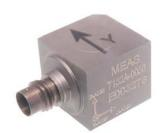
The Model 7132A is a miniature triaxial IEPE accelerometer available in ±50g to ±2000g dynamic ranges. The accelerometer features a hermetically sealed titanium construction with a 4-pin Microtech connector interface. The model 7132A incorporates stable piezo-ceramic crystals in annular shear mode which provide a flat frequency response up to >12kHz.
