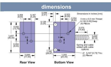
Two through holes and four 3 mm x 0.5 mm threaded holes are provided for mounting.
