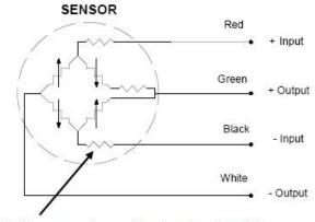
EPL-B0 compensation resistors in external module
