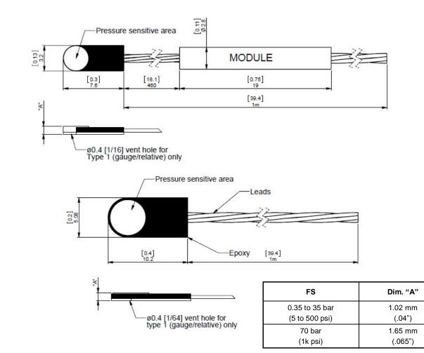
Note : EPL-D1 is internally compensated (no external module) Dim : mm ( inches)
