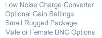
The Model 130 series are remote in-line charge converters designed to be used with piezoelectric accelerometers. The low noise charge converters feature three fixed gain options that convert the high impedance charge output from the accelerometer to a low impedance voltage output. The model 130 series features broad bandwidth to 30kHz and 10Vpeak linear output. The units are powered by a constant current of 4 to 20mA.
