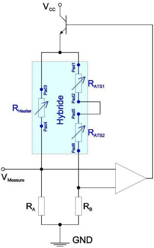
Firgure 3: Outline of a measurement electronics using a Wheatstone-bridge. NOTE: This drawing shows only the basic functionality. This is not a ready to use circuit diagram!
