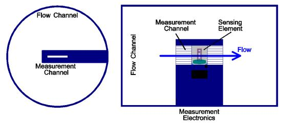
Figure 2: Flow channel of application example of a mass air flow sensor
