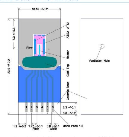
Figure 1: Mechanical dimensions and connections of LMM-H04
